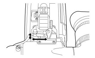
3 Tighten the viewfinder forward-backward/left-right position clamp lever to the locked position.
